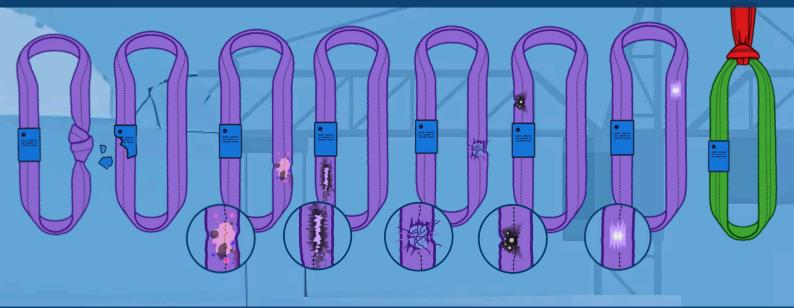
It is tangled or tied, this can weaken the strength of the sling. The tag is missing or illegible. The cover is nicked, this may indicate that the fibers are damaged. Chemical damage is noticeable on the sling. There are holes in the casing - they may have been caused by welding. The casing has damage caused by friction. The core is visible - the fibers in the core may be damaged. It was used with the wrong type of fasteners.
