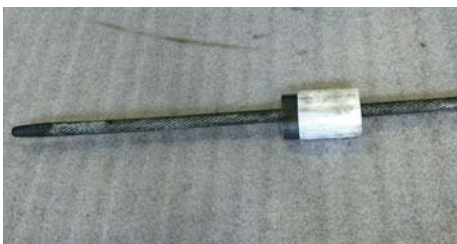
Thread ferrule and T-LOC on wire rope.
