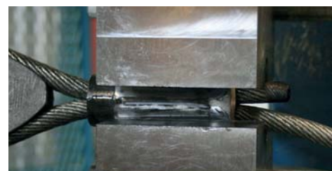
If a second swaging is required, open dies and swage the second part of the ferrule. Close dies. Check the termination to be free from flaws and defects. Diameter and length on the T ferrule should also be checked.
