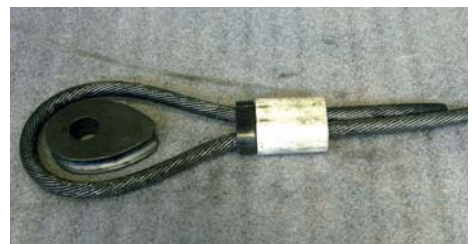
Incorporate thimble, if used. Further adjustment while swaging.
