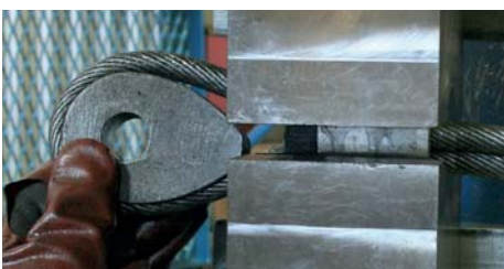
Swage T-LOC and ferrule (or first part of the ferrule, if the assembly is too long for the dies). Close dies. Note! Check alignment during swaging.
