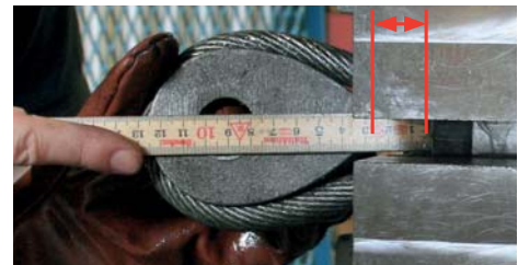
Measure. Distance T-LOC and solid thimble before swaging must be at least 1,5 times the nominal diameter.
